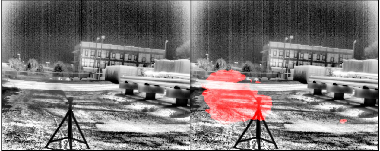
Figure 6: Comparison Showing Good Tracking on Noise Mixed Background; Persistent False Positive Present on Right Side of Image
