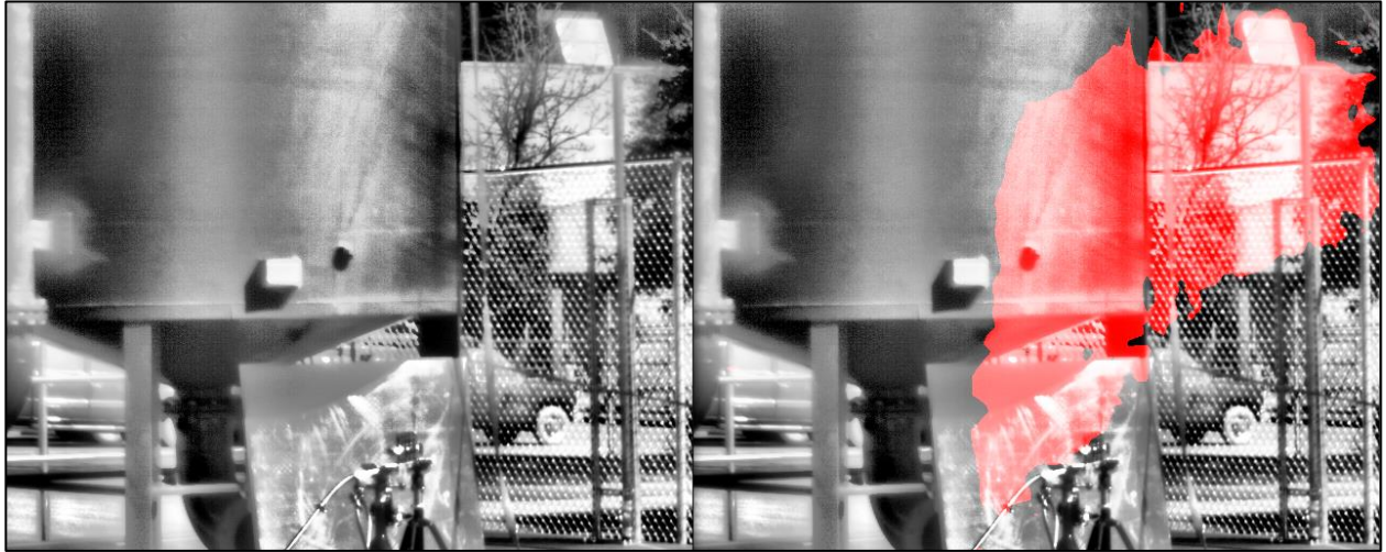
Figure 8: Comparison Showing Good Tracking on Solid Background Again, Failures Present on Bottom-Left of Highlighted Area: Problems Persist Where High-Reflectivity Background Converges with the Plume
