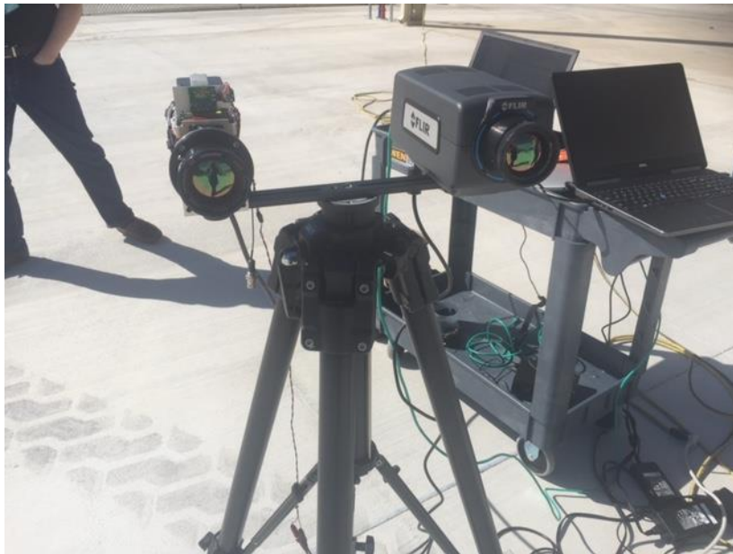
Figure 1: Niatros™ and FLIR MWIR Cameras Acquiring Data During a Supervised Methane Release
