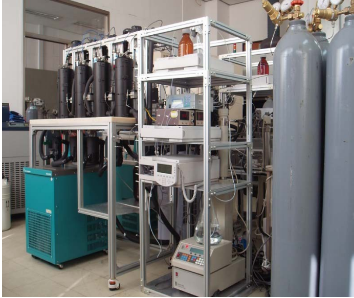
Fig. 2.6. Permeability measurement system of hydrate-bearing sediments
