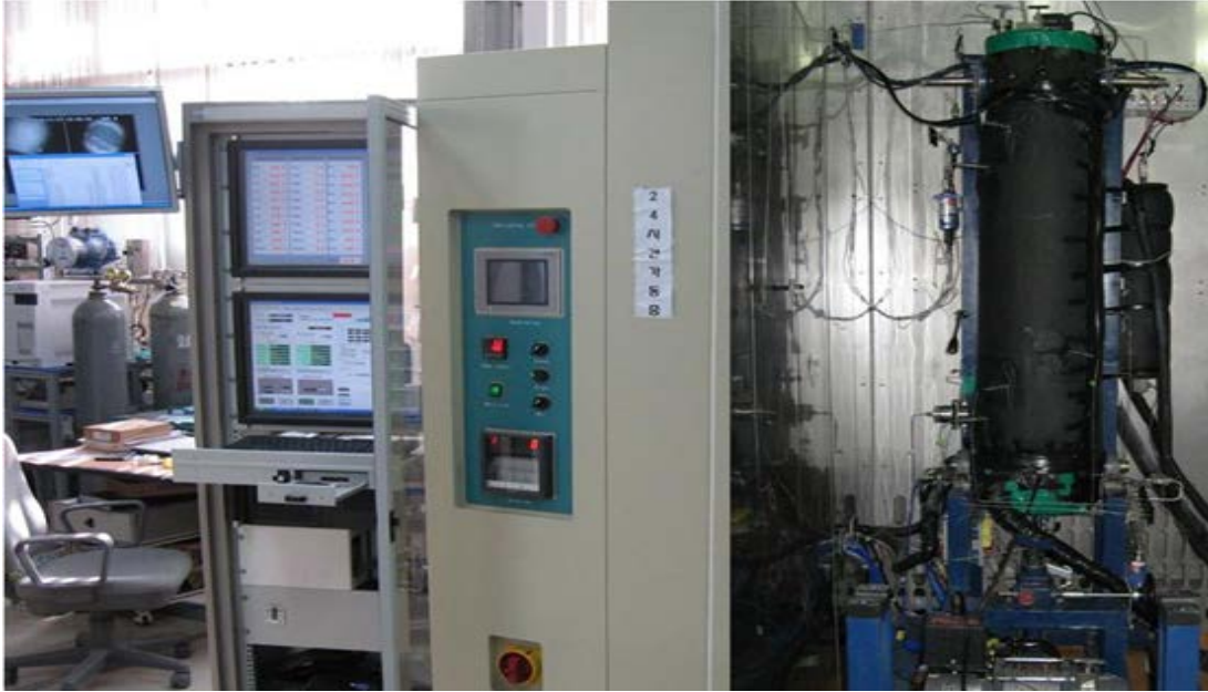
Fig. 2.1. Picture of the experimental setup for 1D 1-m scale GH production
