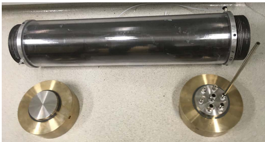
Fig. 3.1. New hydrate pressure vessel with thermal jacket and 2 end caps.
