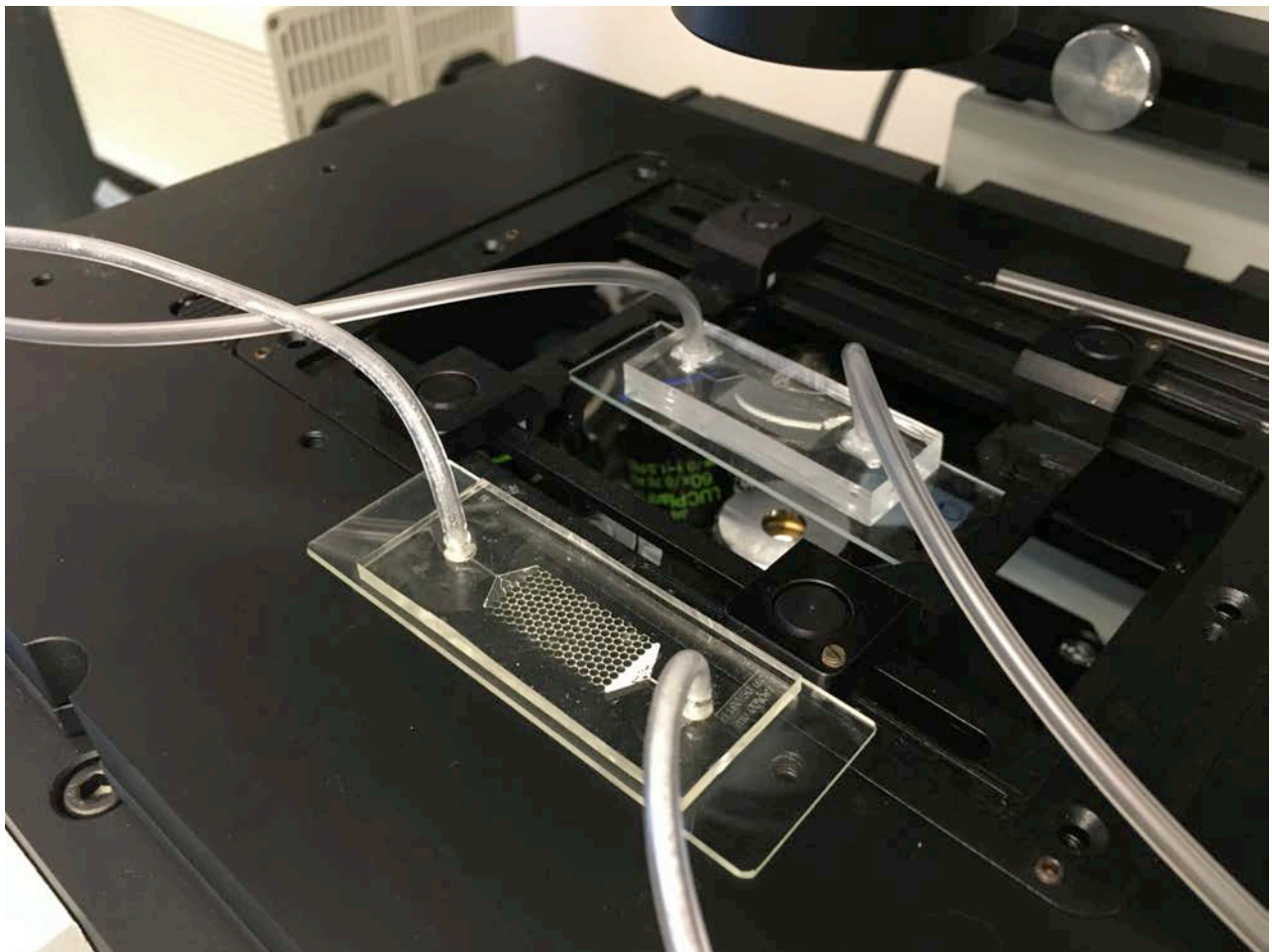
Figure 3: LSU 2D-micromodel observation setup. Two micromodel units, fabricated at LSU, sit atop the microscope imaging stage. A relatively large pore-throat model is in the foreground, with a relatively small pore-throat model in the background. Fluid flow tubes for controlling the inlet and outlet flow have been connected to the units.
