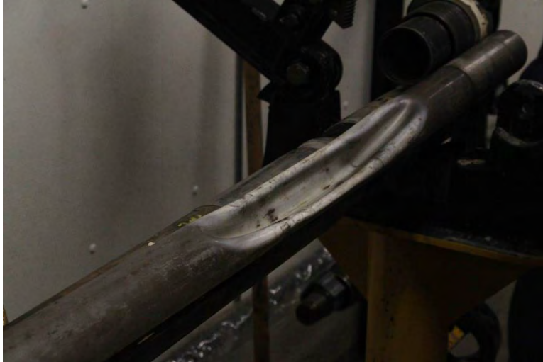
Figure 4: Collapsed liner after Flow Test 3.
