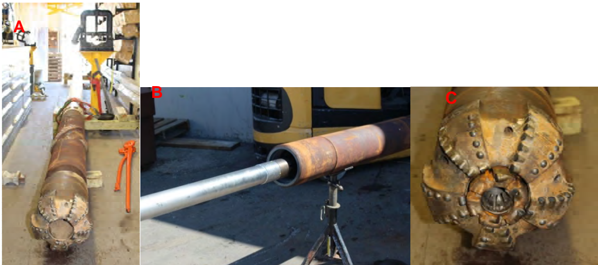
Figure 5: Horizontal space-out test. A) The bottom hole assembly viewed from the bottom. B) The PCTB inserted into the head and top sub. C) The face bit with cutting shoe fully inserted.
