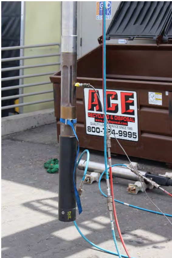
Figure 1.3: Lower end of PCTB with ball valve capped and annulus filled with water and pressurized
