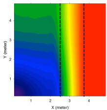
Due to the dominancy of x-direction permeability, flow is almost horizontal. The low permeability in the mud layer prevents the invasion of the flow. Only very few tracer flows across the mud layer and enters the sand to the right.
