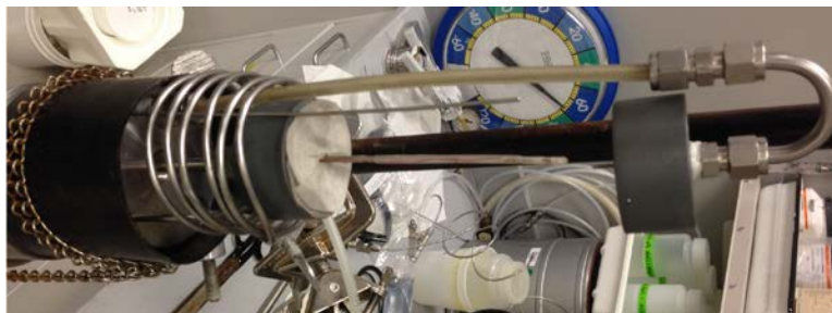
Figure 6. Temperature adjustment coils (left) located around the base of the sample inside the pressure vessel.
