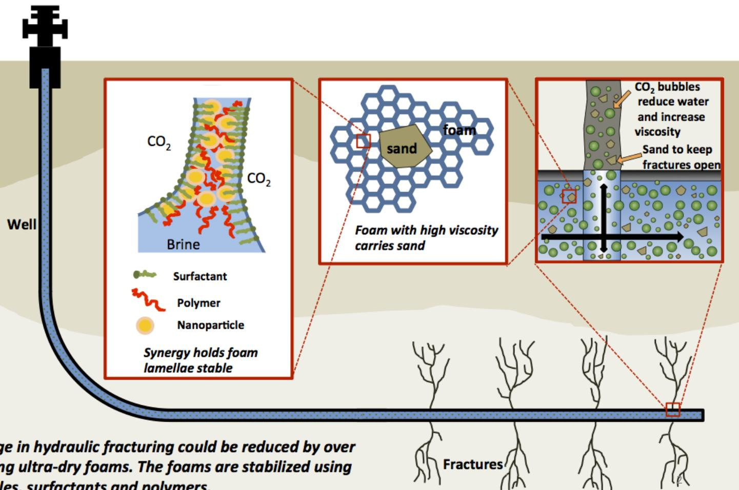
*Water usage in hydraulic fracturing could be reduced by over 90% by using ultra-dry foams. The foams are stabilized using nanoparticles, surfactants and polymers.*
