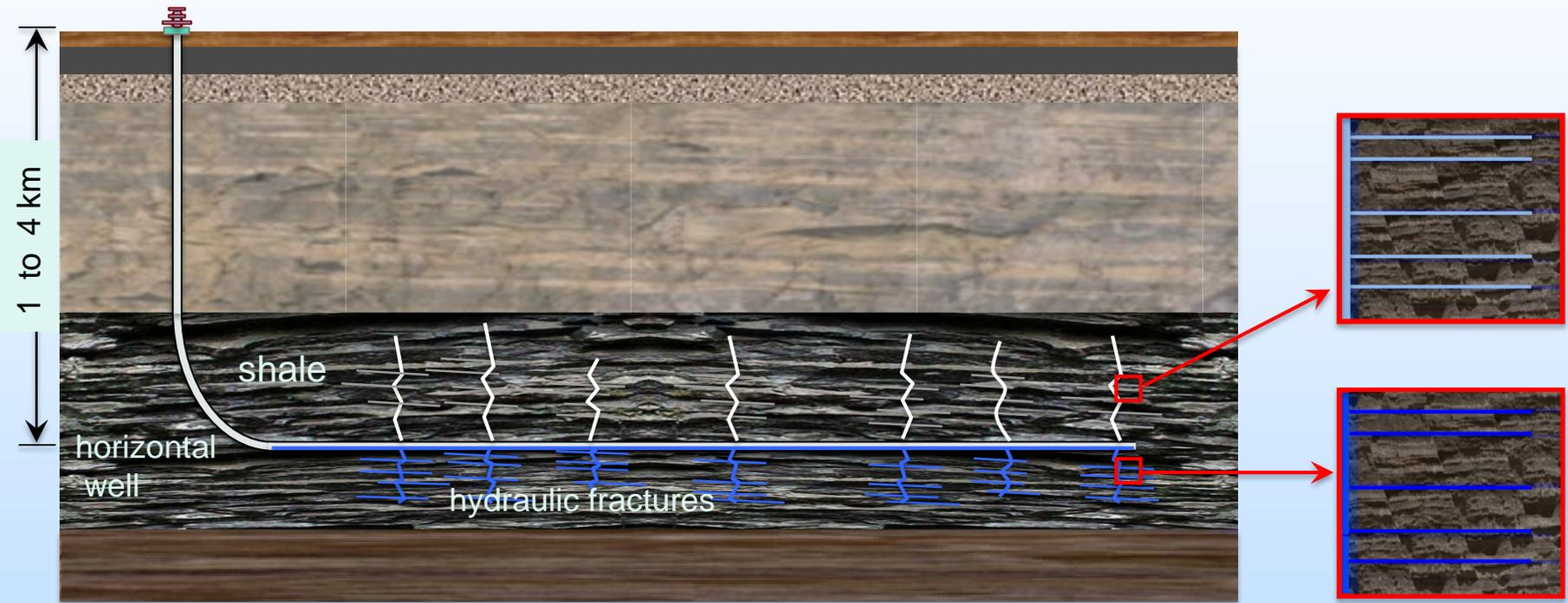
In addition, natural and stimulated secondary horizontal fractures connected to primary, above-well fractures should more easily drain.
