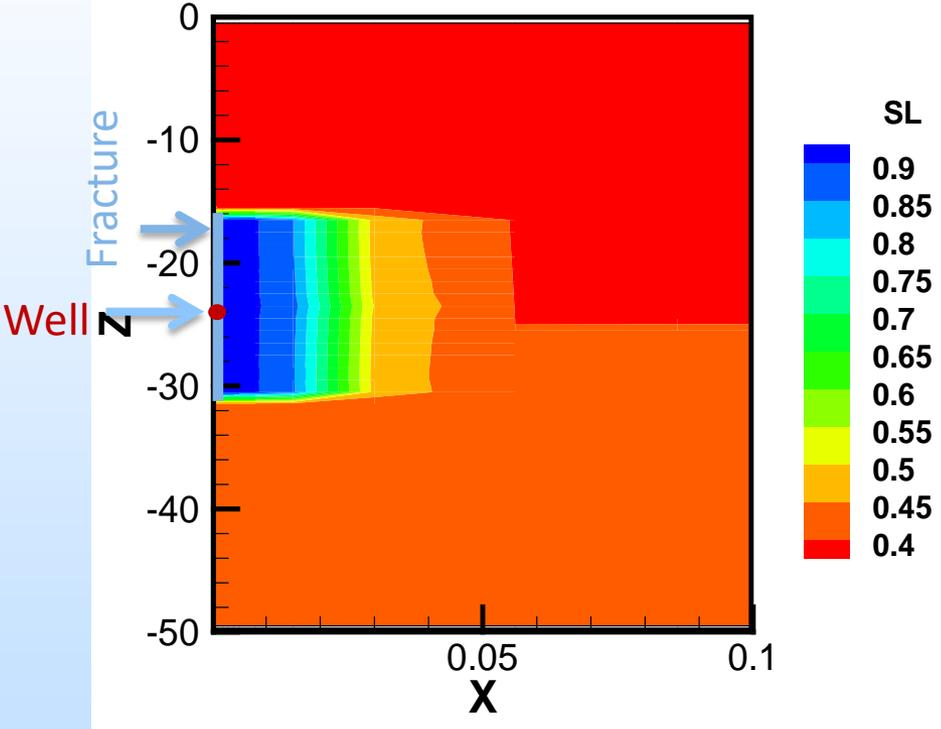
Liquid saturation after 2 hours of injection
