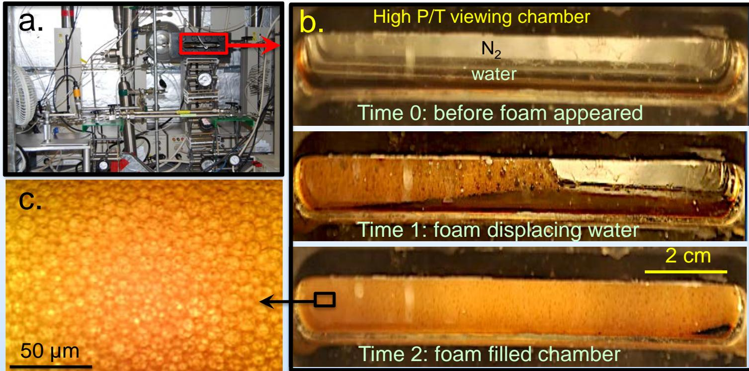
(a) Photo of foam generator and rheometer for supercritical fluid foams
