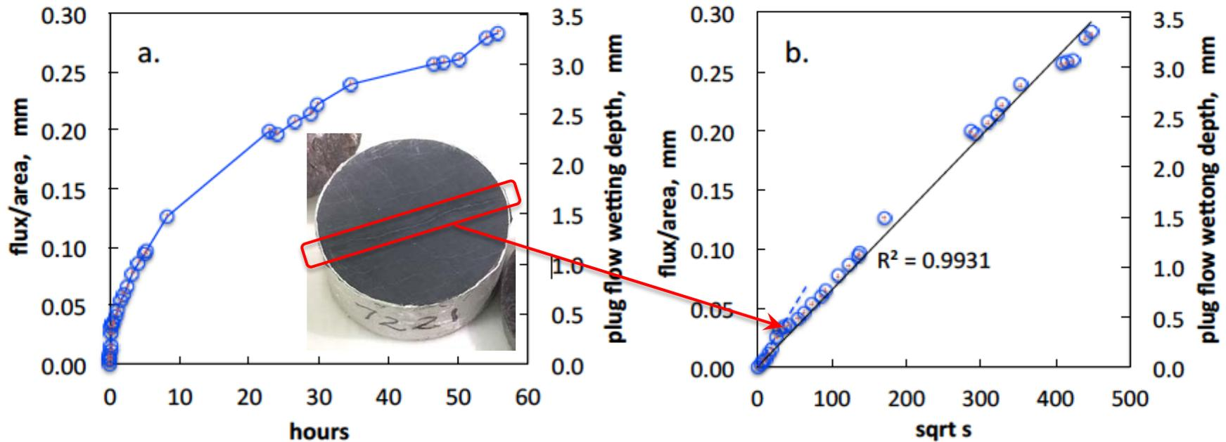
Water (1 M NaCl) imbibition into Marcellus Shale (7221') at 23 °C, and atmospheric P. (a.) Volumetric influx per unit core area, with through-going microfracture framed in photo. (b.) Square-root of time water uptake plot, showing **initial rapid flow into microfracture** (dashed trend line).
