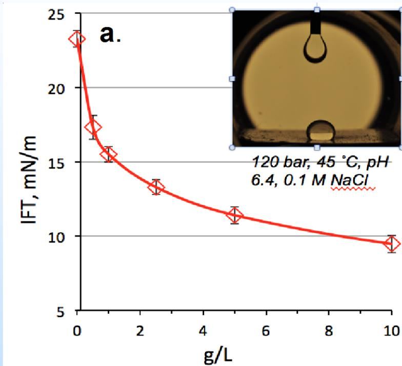
(a) Image of equilibrium NBS solution droplet within scCO<sub>2</sub> at 12.0 MPa and 45°C. The IFT values were calculated from the image.
