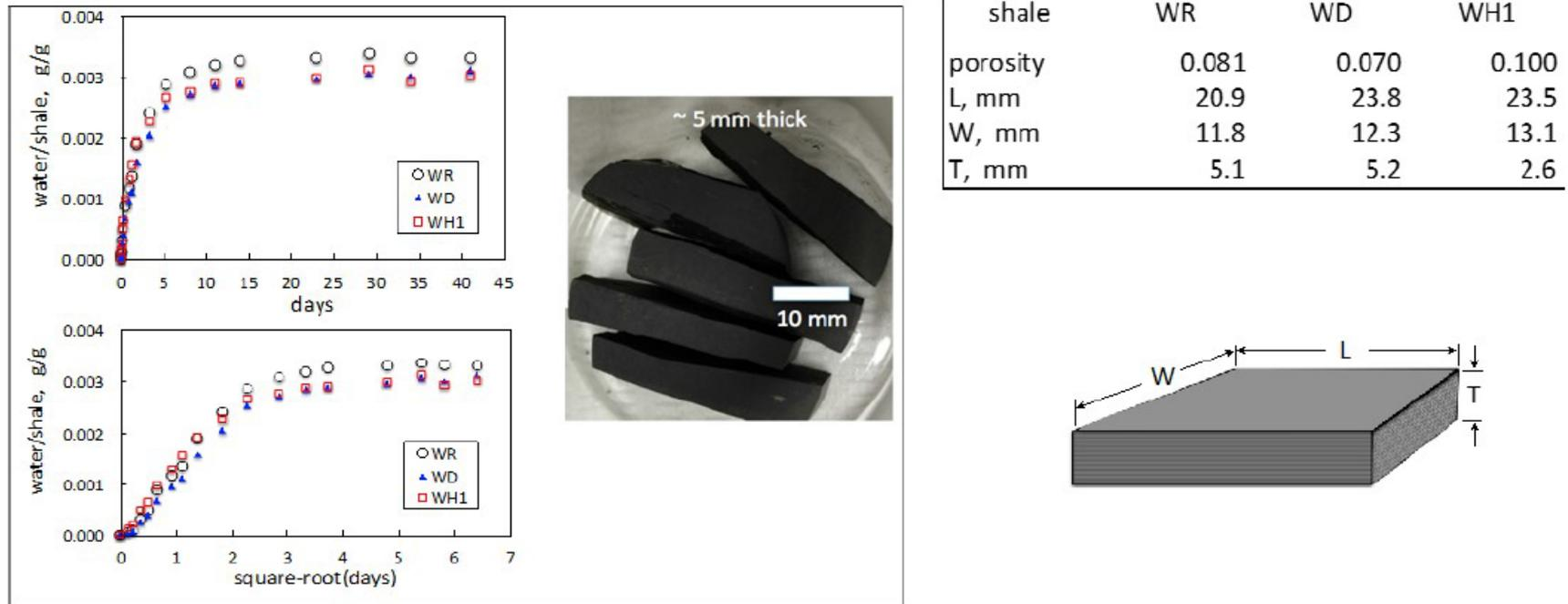
**Figure 5.** Average equivalent rectangular parallelepiped dimensions of the shale rock blocks and the results of the water molecule uptake experiments through diffusion and adsorption.
