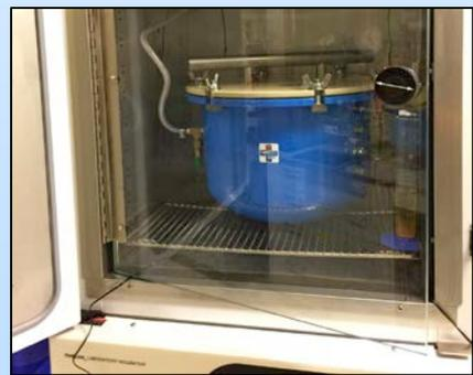
0.5 MPa pressure-plate system in  $50^\circ\text{C}$  incubator
