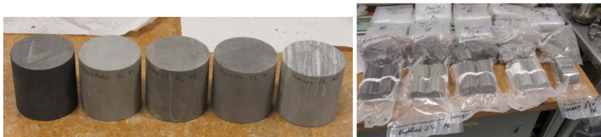
Figure 2-5 Five types of shale samples (From the left, Barnett, Niobrara, Eagle Ford, Marcellus, and Mancos shales) used in our current experiments.
