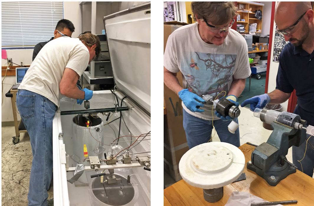
Figure 2. Left: The conductivity cell installed in the Menlo Park gas hydrate laboratory. Right: Removing the sample after quenching in liquid nitrogen.
