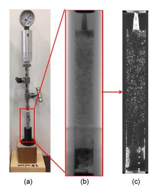
Figure 1. (a) Hydrate experiment set-up picture, (b) X-ray radiography image of the  $k_o$  pressure vessel at 38 days (resolution = 49.79 um, dark color is hydrate or stainless steel), and (c) micro CT image slice of the  $k_o$  pressure vessel at 38 days in orthogonal view (resolution = 49.79 um, white color is hydrate or stainless steel)
