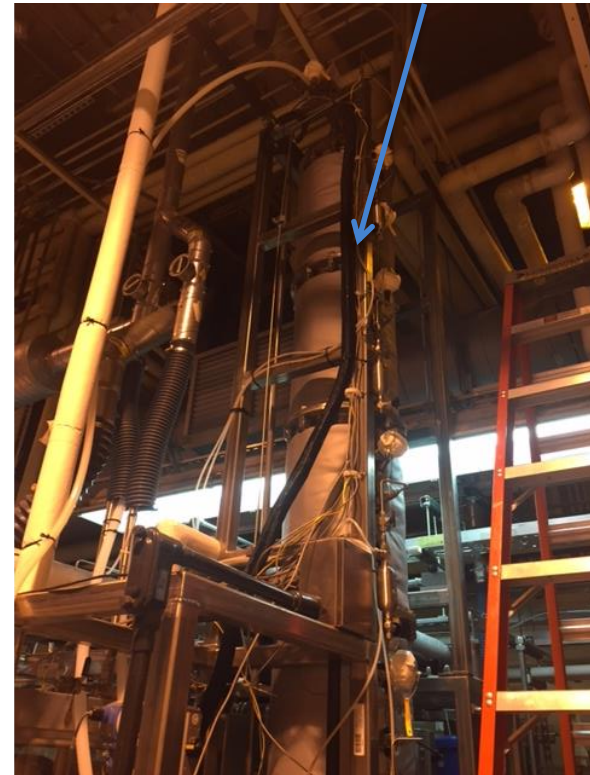
Heated FTIR Line – Top of the absorber
