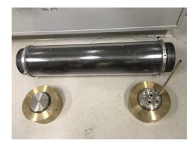
Task 11. Assessment of thermal gradient modification methods and Investigation of the effect of thermal gradient and gradient oscillation on hydrate behavior – We are designing methods to temperature gradient application. We are investigating the use of viscosity adjustment chemicals (gelatin) to reduce fluid convection and found the correct formula resulting in the proper viscosity, the use of
