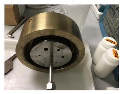
Tests this quarter were performed in the older vessel because of sealing problems with the cooling jacket on the new vessel. These problems required redesigning the cooling jacket and modifying the application of the jacket. A weak gelatin was used as the confining fluid to improve conductive heat transfer, and temperature measurements were made using a sliding thermocouple in a Teflon fitting.
