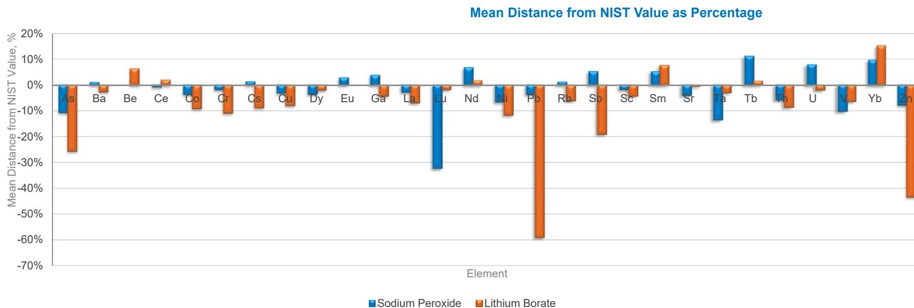
Comparison of Sodium Peroxide vs. Lithium Borate digestion using NIST sample
