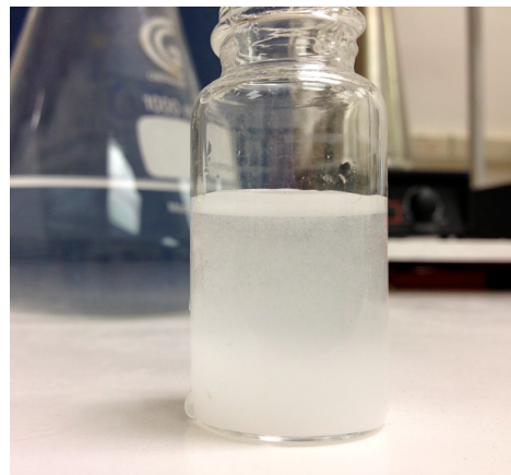
Figure 5. Precipitants clearly visible in FGD Concentrate.
