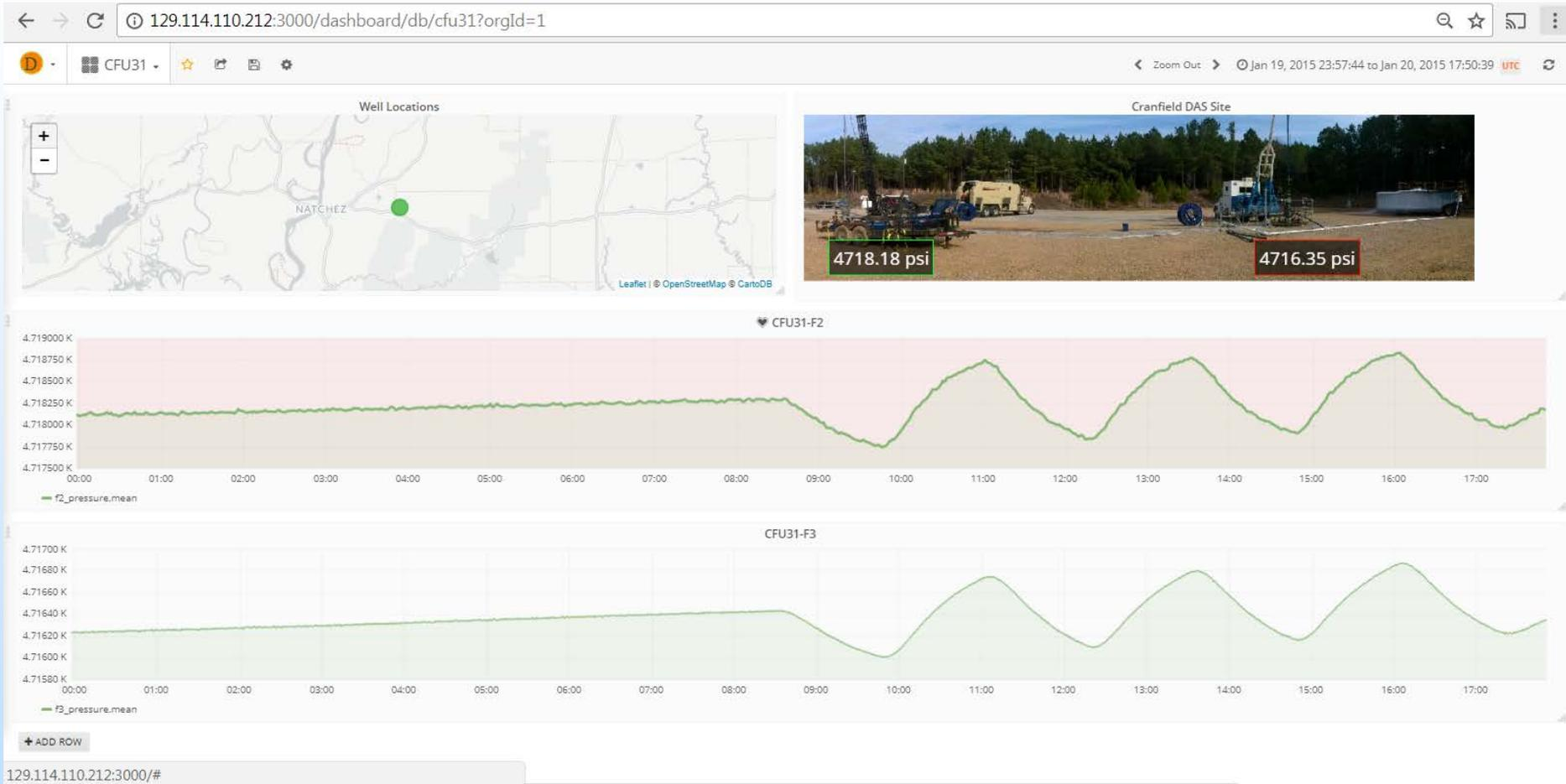
Data collected during simulated leakage field test at Cranfield, MS
