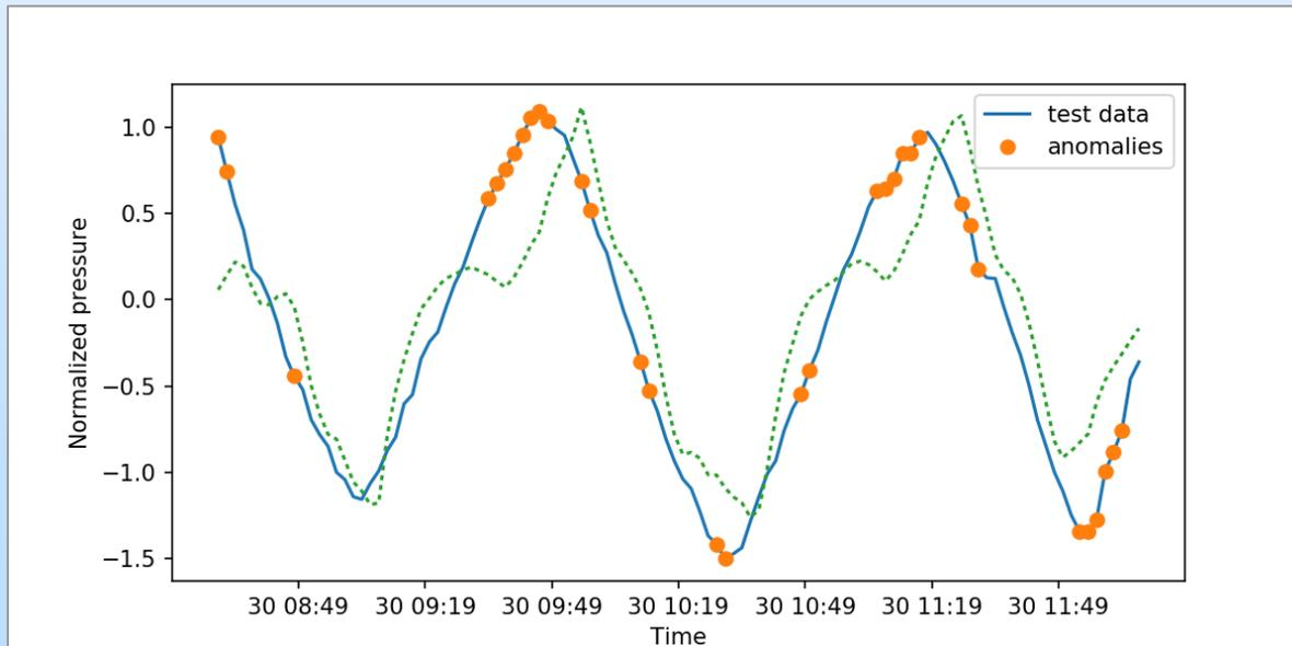
***Leaks caused phase and magnitude deviations from the predictive model***
