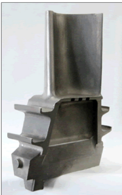
A single-crystal model blade (length:170mm).
