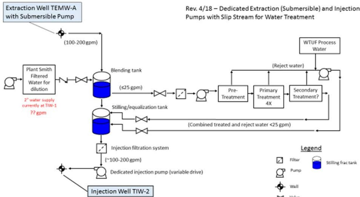
Flow diagram showing major components of the EPRI water treatment user facility
