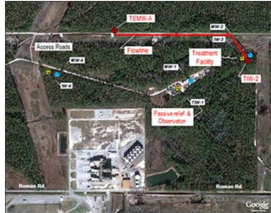
BEST project infrastructure layout showing the proposed location of the extraction well (TEMW-A), injection well (TIW-2) and flowline, and the existing passive-relief well (TIW-1)
