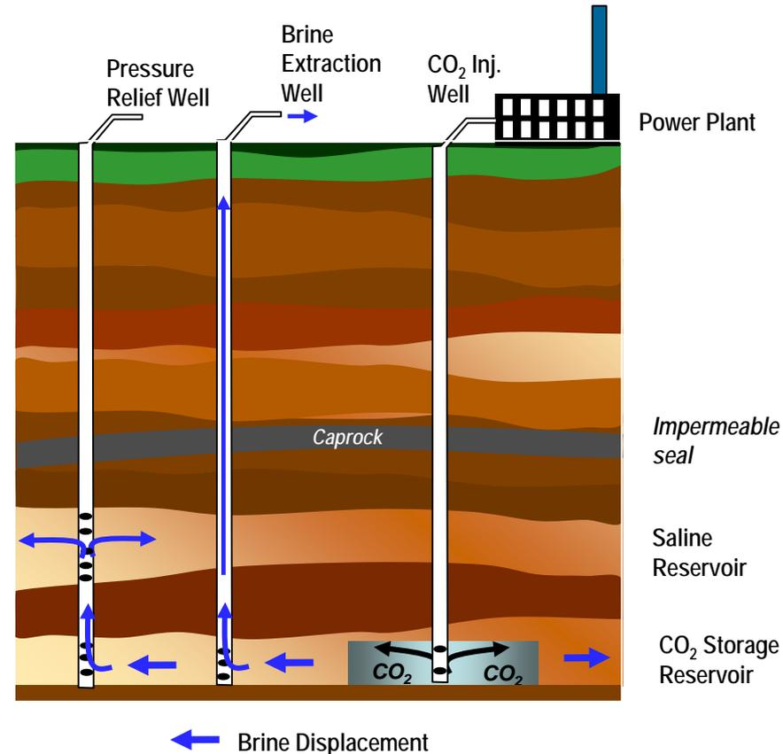
Hypothetical CO<sub>2</sub> storage project showing “active” extraction and “passive” pressure relief well
