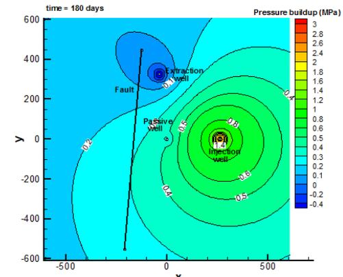
Addition of extraction well reduces pressure on a hypothetical fault (line)
