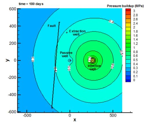
Pressure distribution from active injection & passive pressure relief
