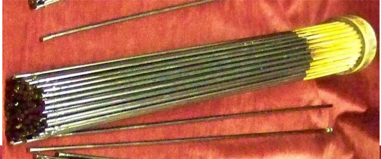
*Pd-Alloy Multiple Tube Bundle with Full Ceramic Tube Sheet*
