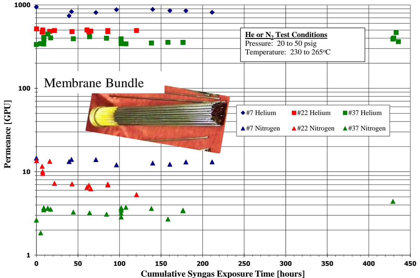
*Performance stability of multiple tube CMS membrane bundles during H<sub>2</sub> recovery from NCCC slip stream testing. He and N<sub>2</sub> Permeances measured periodically during >400 hr test.*
