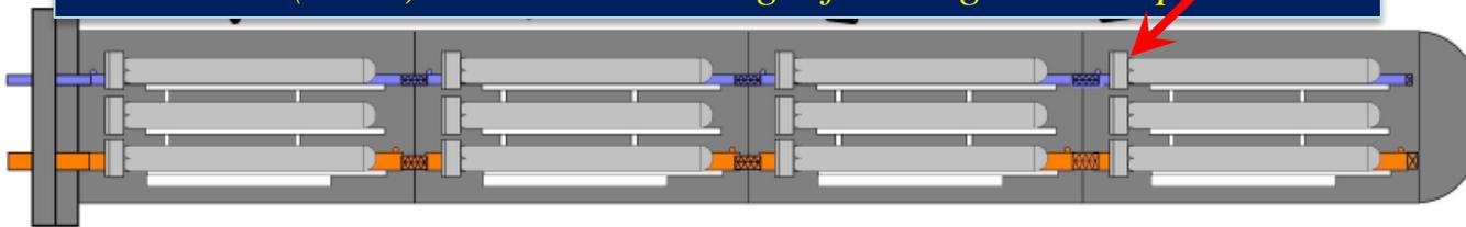
Total Pressure Jacket Length 200" of 24" Pipe, 4 sections of 7 Bundles connected with flexlines.
