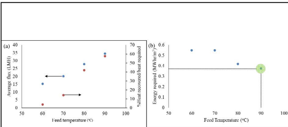
(a) Average flux and percent heat recovery vs Feed Temperature
