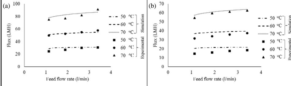
Flux vs flow rate at 50, 60 and 70 °C for (a) 93 g/l and (b) 308 g/l TDS produced water solutions
