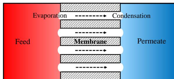
Schematic diagram of liquid/vapor interface across a hydrophobic membrane
