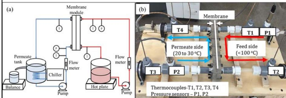
(a) Schematic diagram of experimental setup,
