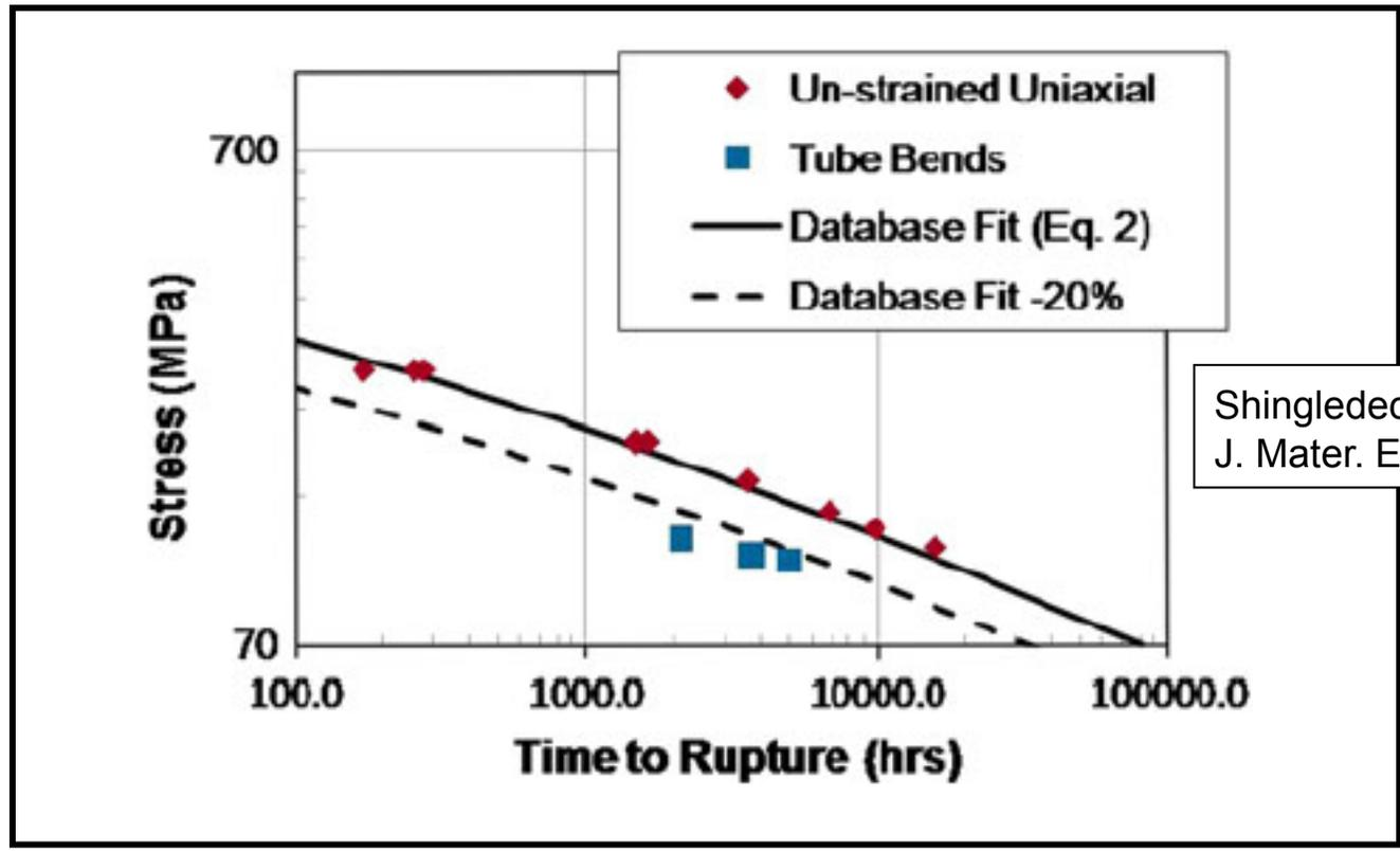
*Creep rupture of solid-solution Ni-based alloys thought to be less susceptible to cold work effects than precipitation-strengthened alloys such as Inconel 740*
