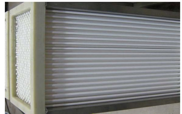
TMC tubes in a bundle assembly
