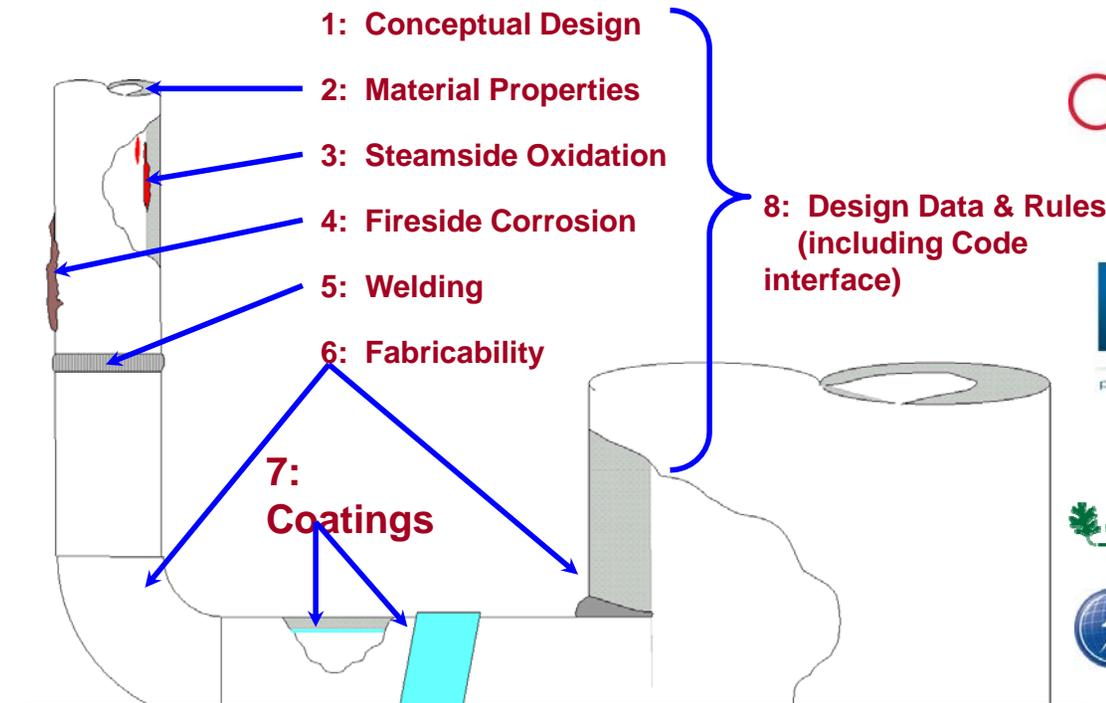
**Develop the materials technology to fabricate and operate an A-USC steam boiler with steam parameters up to 1400°F (760°C)**
