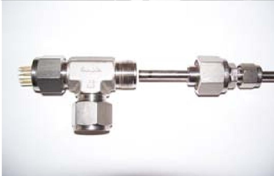
**Sensor mounted 16 pin transistor outline header with microheater & RTD for temperature control & readout (Temperatures  $\leq 800$  °C)**
