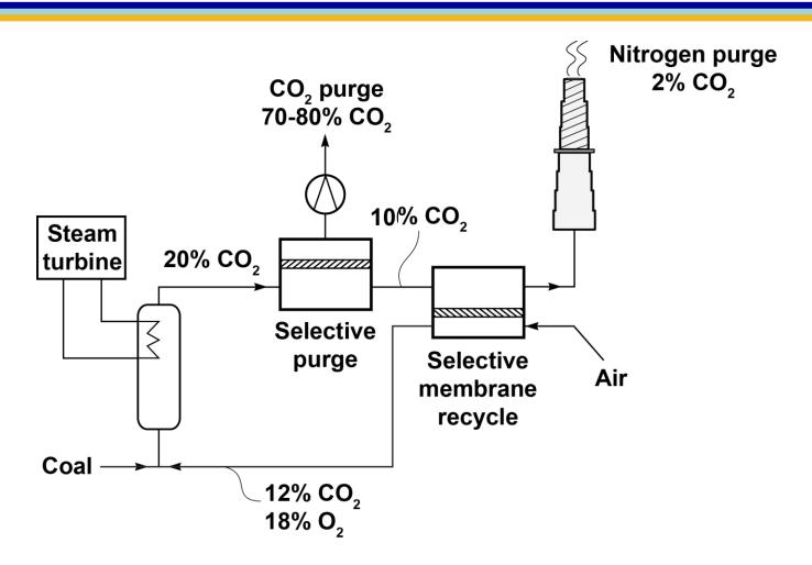
500 MW<sub>e</sub> plant requires one million m<sup>2</sup> of membrane
