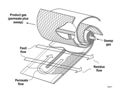
Each module contains 20 to 50 m<sup>2</sup> of membrane
