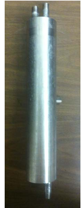
Module for lab testing (Ø2" x 15" long, 0.5m 2 )
