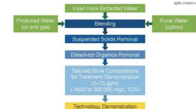
*Conceptual extracted water pretreatment flow diagram.*
