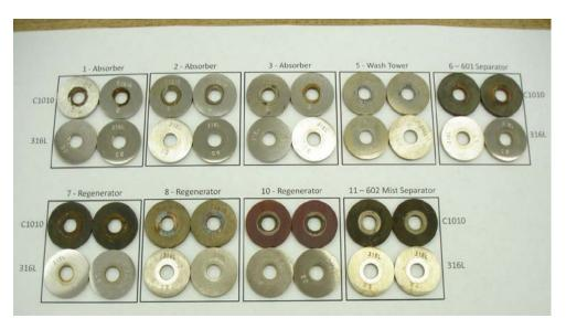
• Coupons installed throughout the PSTU to assess how corrosion rates of different materials vary with location.
