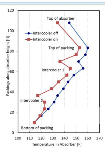
Operation with intercoolers raised capture efficiency 6 percentage points (90 to 96%)  PSTU can gather solvent density, viscosity, and specific heat data for a range of CO<sub>2</sub> loadings to validate and/or expand physical property database.
