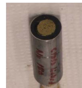
Potted fiber bundles with 14-in length, 100 fibers, and high packing density
