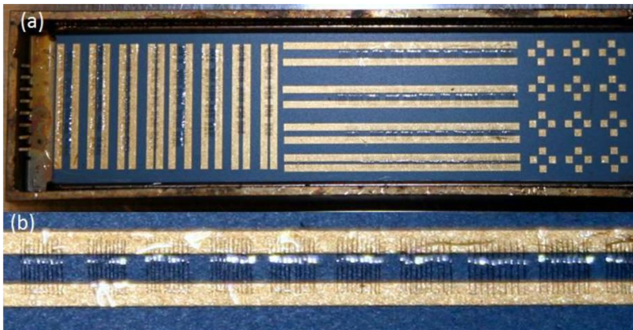
Figure 37: Completed Bond Test Board (a) and a Close-up View of the Bonds (b)
