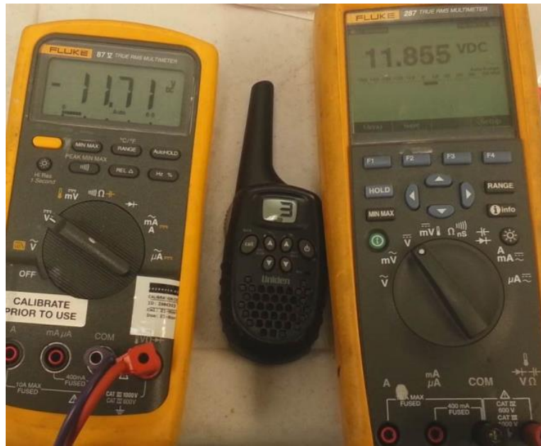
Figure 59: Monitoring of Rectified Voltage on Spinning Electronics Board
