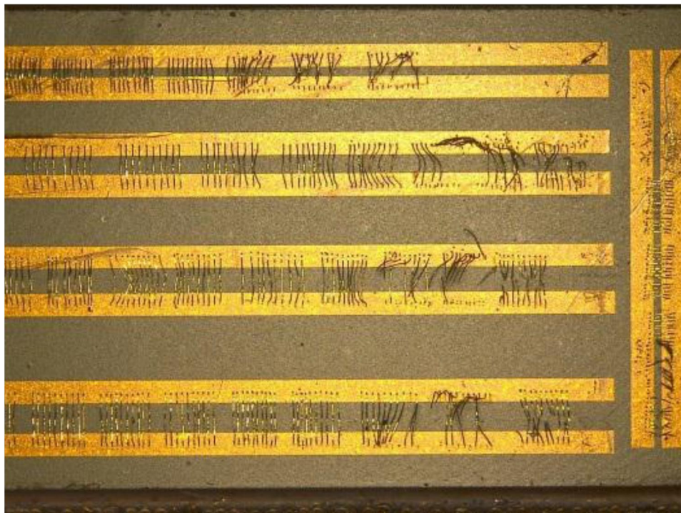
Figure 39: Board 3 after 20 Thermal Cycles at 450°C
