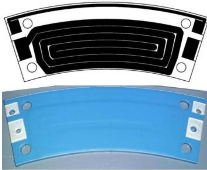
Figure 76: Internal Diagram and Photo of LTCC Magnetic Coil Arc
