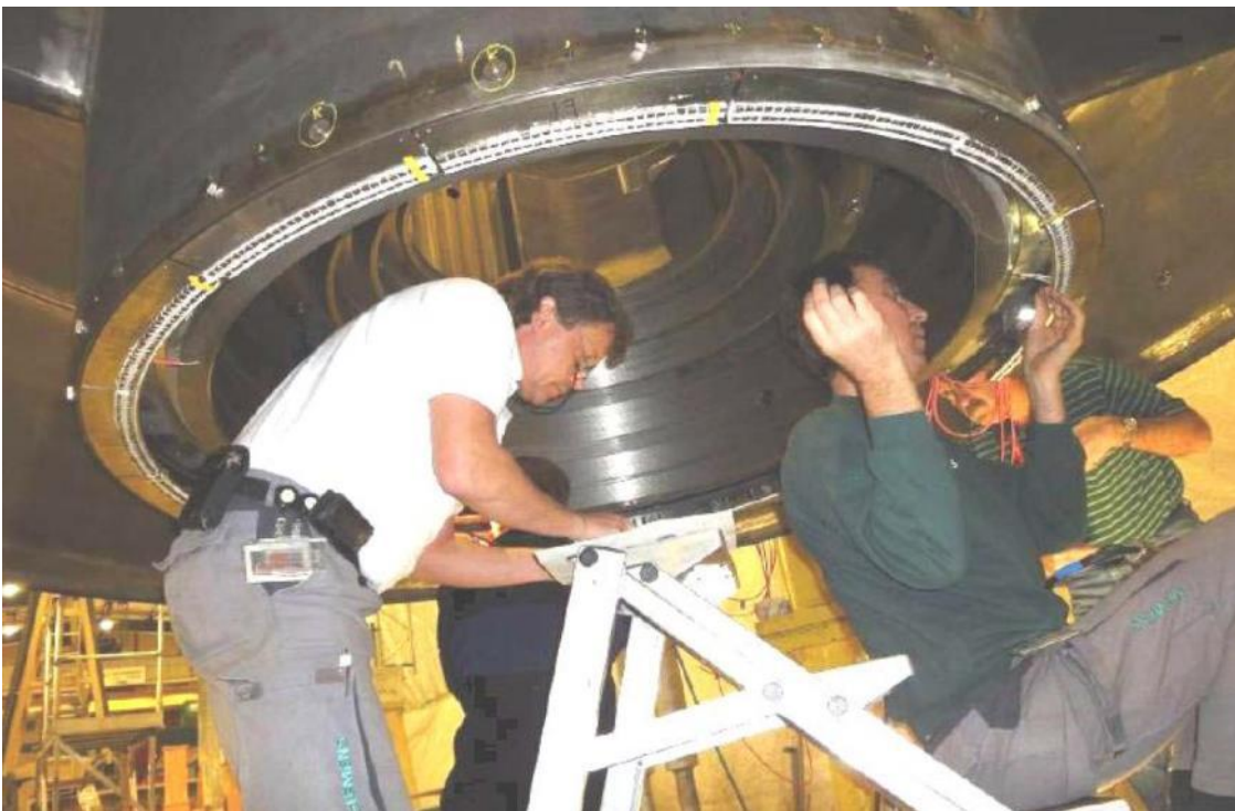
Figure 69: Stator Ring Installation in H-Class Engine
