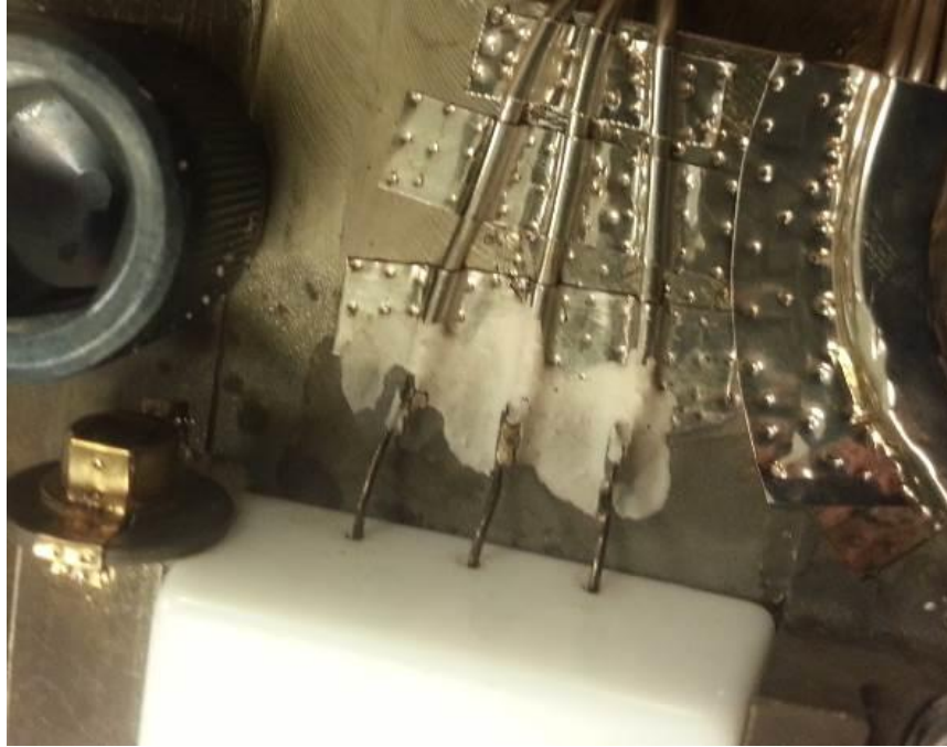
Figure 115: Rotating Antenna Pins after Spin Test
