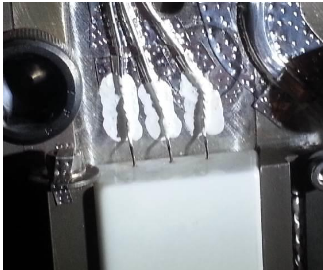
Figure 112: Rotating Antenna Pins before Spin Test
