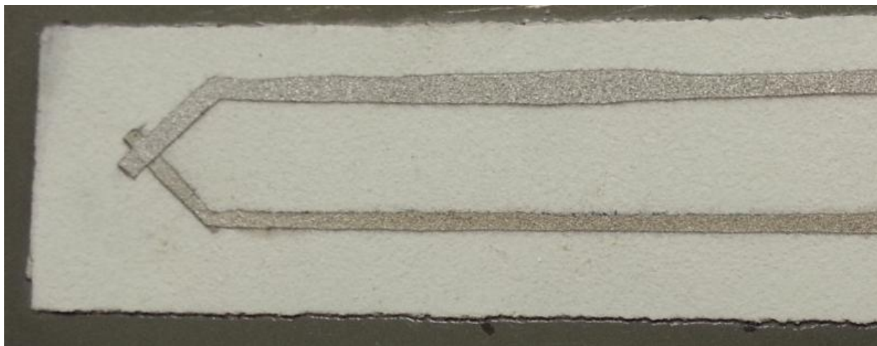
Figure 30: Close-up of Spray-On Thermocouple Applied to H-Class Blade
