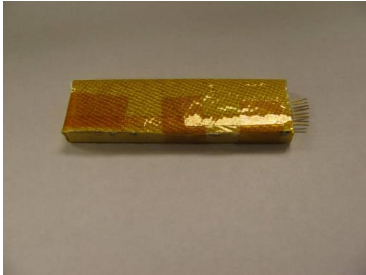
Figure 15: Electronics Board Wrapped in Alumina Mesh and Tape
