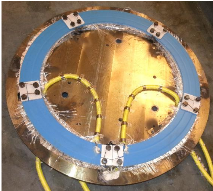
Figure 116: Inductive Power Ring after Spin Test
