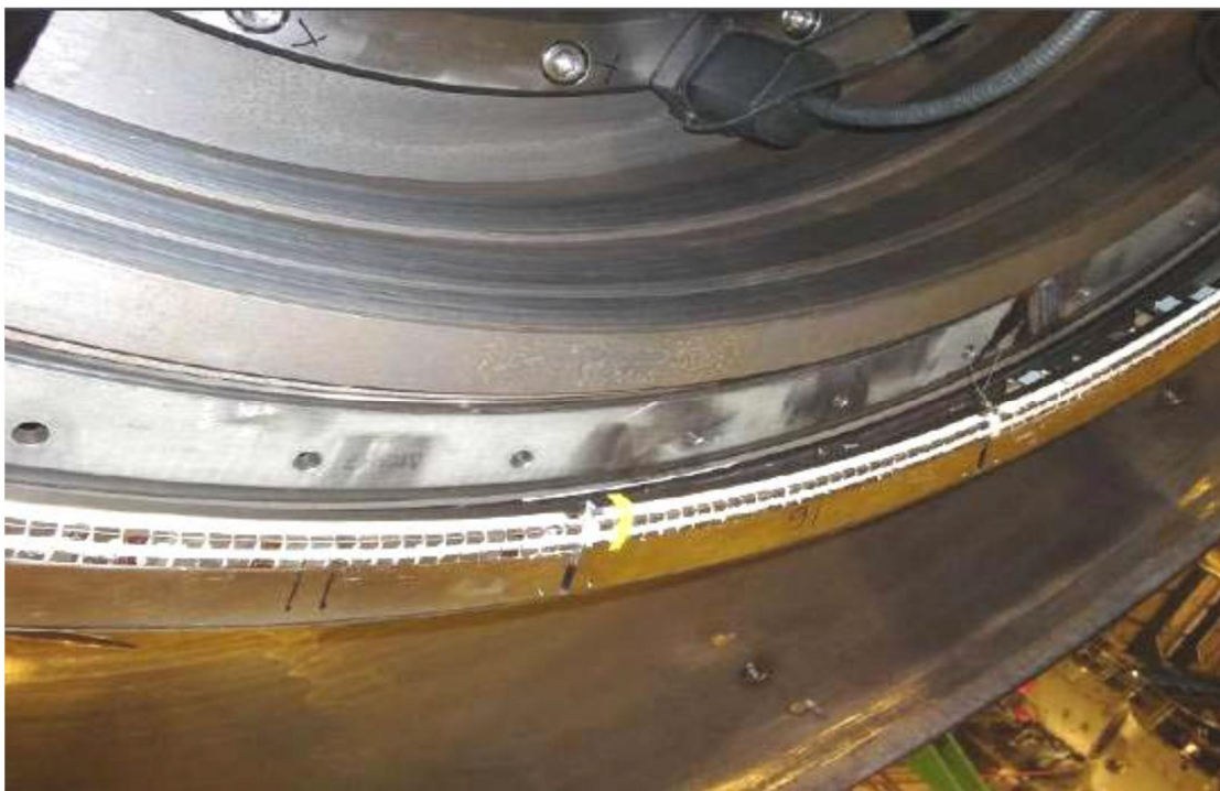
Figure 70: Stator Segments Installed in H-Class Engine
