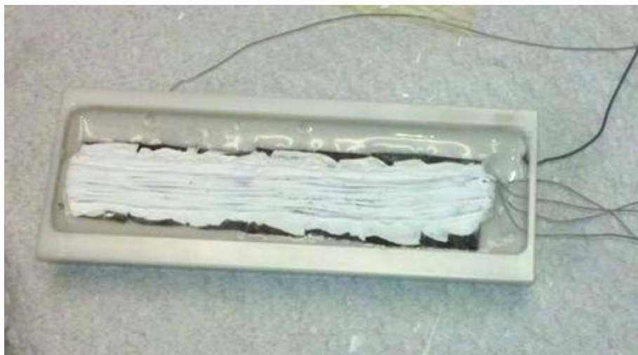
Figure 80: Wound Core Assembly Potted into the Ceramic Box
