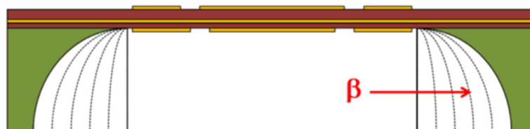
Figure 124: Sidewall Etching Angles Under a SiC Pressure Transducer
