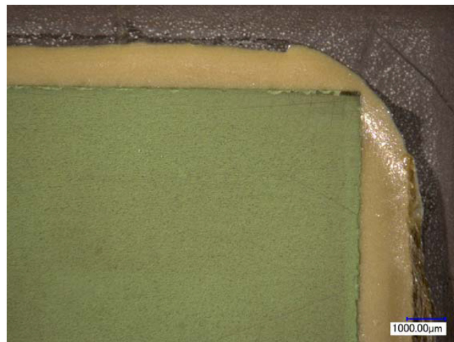
Post-test image of SCN-1 compliant glass sealed between aluminized AISI441 and an anode/electrolyte bilayer. No evidence of damage or leakage was observed after 12 thermal cycles between RT and 800 °C.
