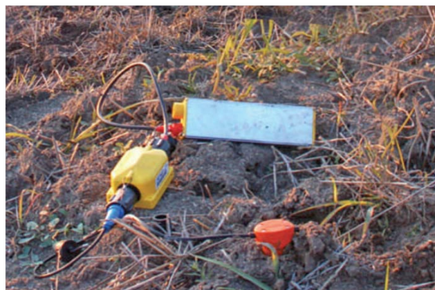
Figure 1. Surface receiver unit to be deployed as part of the SASSA package. The surface receiver gathers seismic reflection data from the source instrumentation located in the subsurface.
