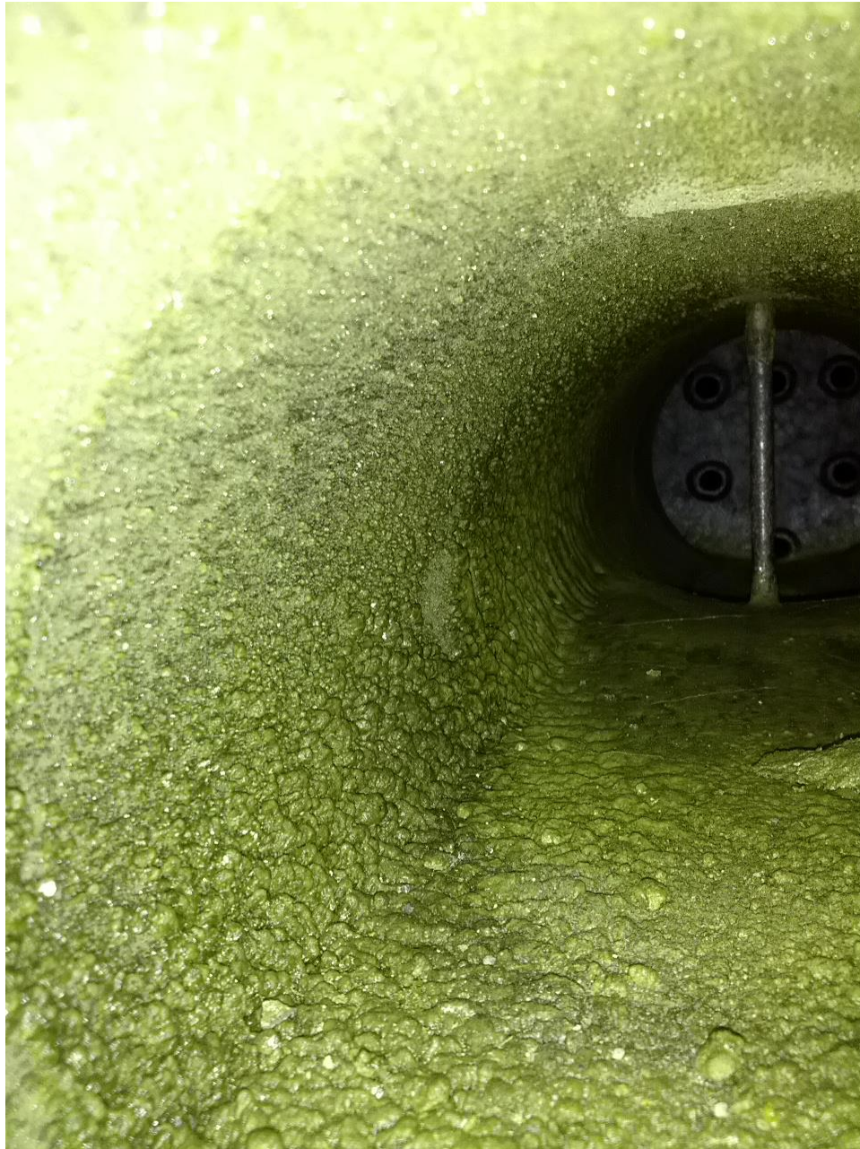
Figure 49. Close-up view of sulfur in outlet plenum of reactor intercooler HX-04.
