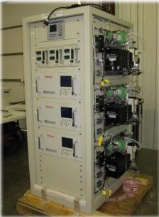
CEMS Gas analyzer measures O<sub>2</sub>, CO<sub>2</sub>, CO, SO<sub>2</sub>, NO, and NO<sub>2</sub>
