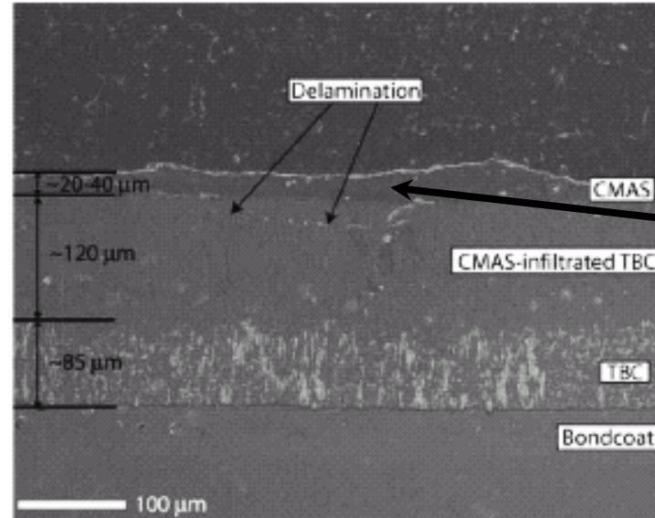
Transverse Cracks that Lead to Shedding of Topcoat
