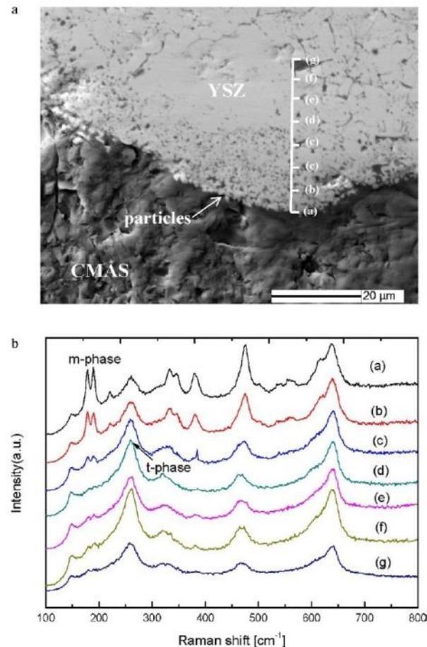
Fig. 4. (a) Micrograph of the interaction zone of CMAS deposit and YSZ coating after 4h heat-treatment at 1250 °C, and (b) Raman spectra obtained from the positions marked in (a).
