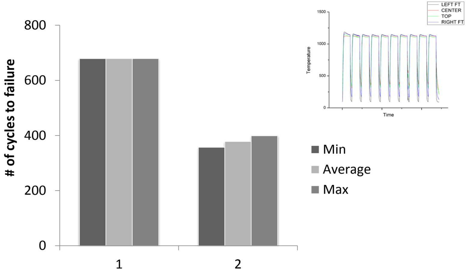
Cyclic furnace testing of: (1) 250 μm SPPS YSZ with IPBs, and (2) 250 μm APS YSZ.
