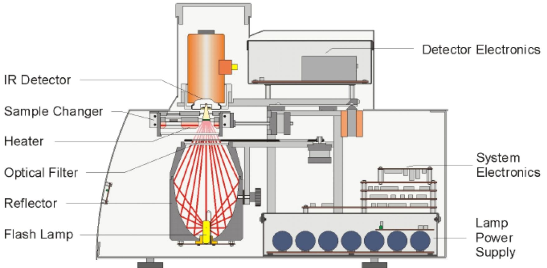
Figure 2: Schematic of the NETZSCH LFA 447
