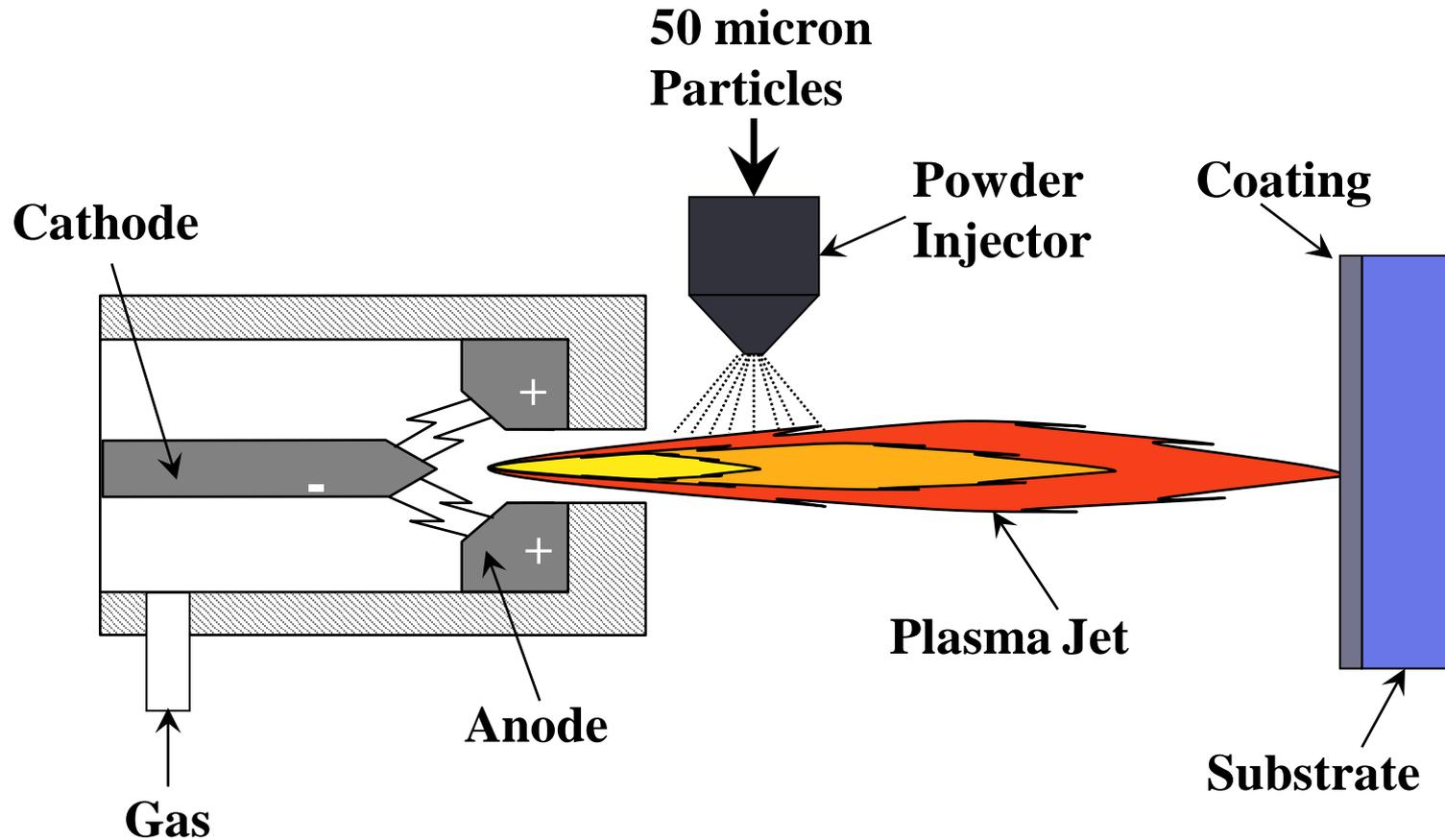
Particles melt and form splat structures → 7YSZ
