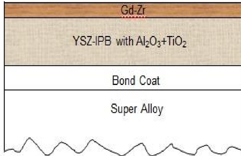
**TBC system #2 with low conductivity solution plasma sprayed YSZ with IPBs and CMAS resistant high temperature tolerant GdZr protective surface layer (PSL).**
