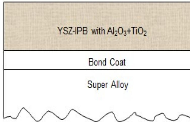
**TBC system #3  $\text{Al}_2\text{O}_3/\text{TiO}_2$ -doped SPPS YSZ TBCs
