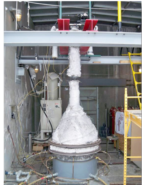
Figure 3. OSU turbine reacting flow rig (TuRFR) showing upper and lower sections assembled.
