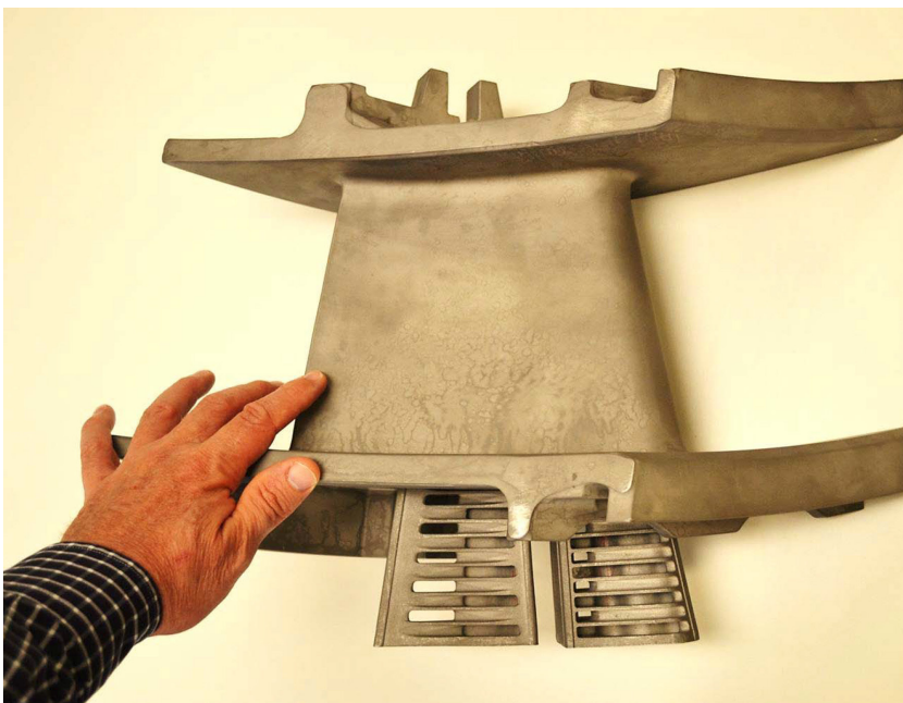
FTT Spar-Shell Vane under Construction for Test in a Large-Scale Industrial Gas Turbine Engine.
