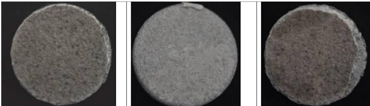
Figure 2. (L) YSZ, (M) GZ, (R) 50%GZ/YSZ, Failed TBC samples after thermal gradient thermal cycling tests. Failure is mainly caused by the spallation at the edges.
