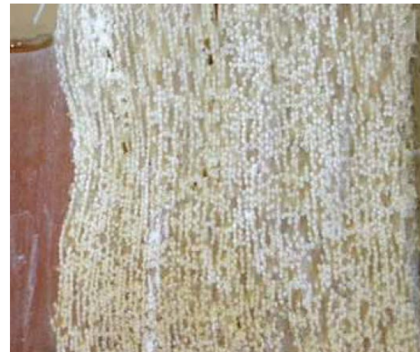
Tubesheet with good fiber epoxy adhesion
