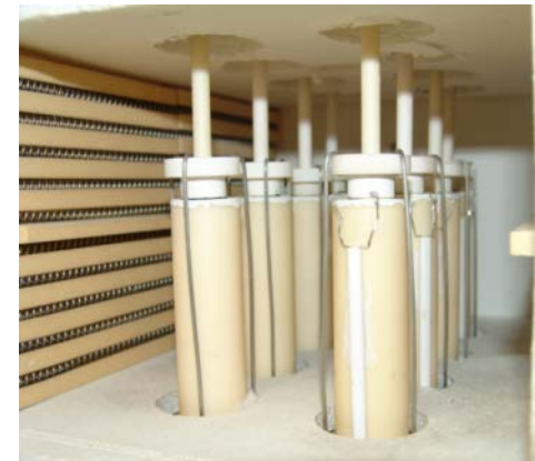
Multiple button cells per furnace with individual gas flow and electrical control
