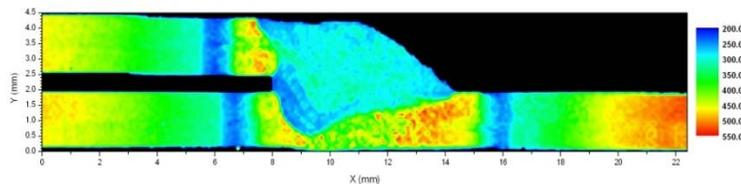
Simulation of HAZ softening of a boron steel
