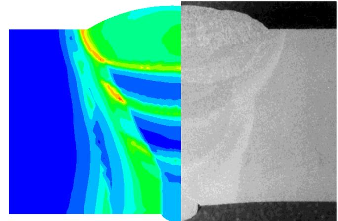
Yield strength gradient simulation in a multi-pass steel weld
