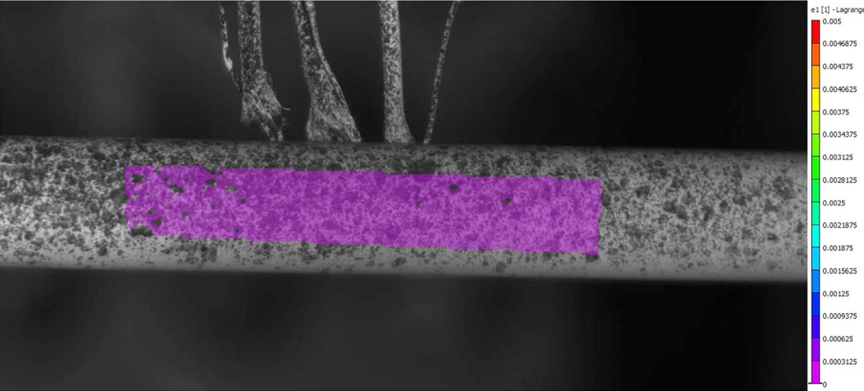
Significant strain concentration is shown after **30** hours of test
