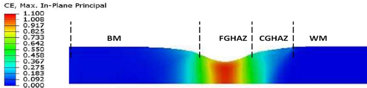
Figure 1. Maximum in-plane creep strain in a cross-weld specimen after 13000 hours creep. (CE is in-plane principal creep strain)
