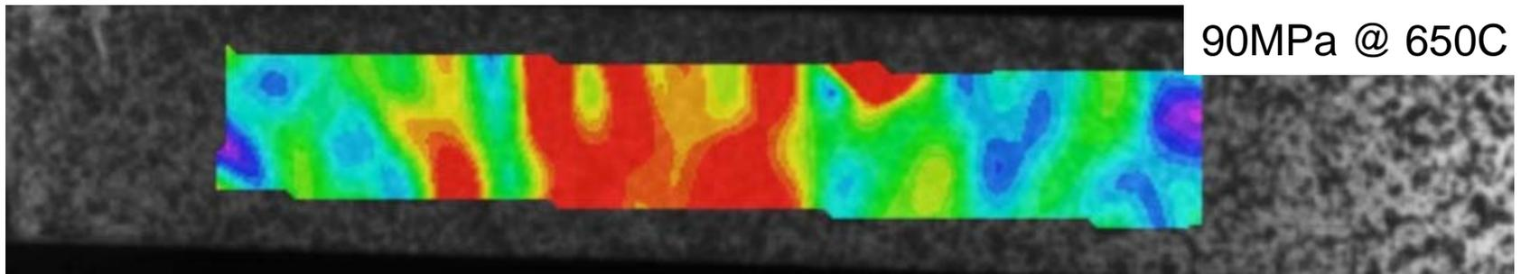
Strain rate can be extracted from each individual location
