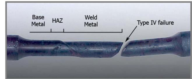
Weld Joint Strength Reduction Factors ( $WSRF = \sigma_{weld} / \sigma_{base\ metal}$ ) for CSFE steels can be as low as 0.5 at  $-600^{\circ}C$ .
