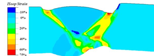
Performance simulation of a high strength steel weld
