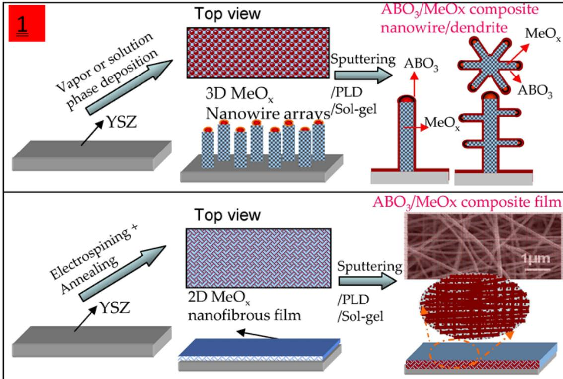
MeO<sub>x</sub>: metal oxide semiconductor, demonstrated in industry sensing up to 700°C. → can we improve the temperature range and functionality?
