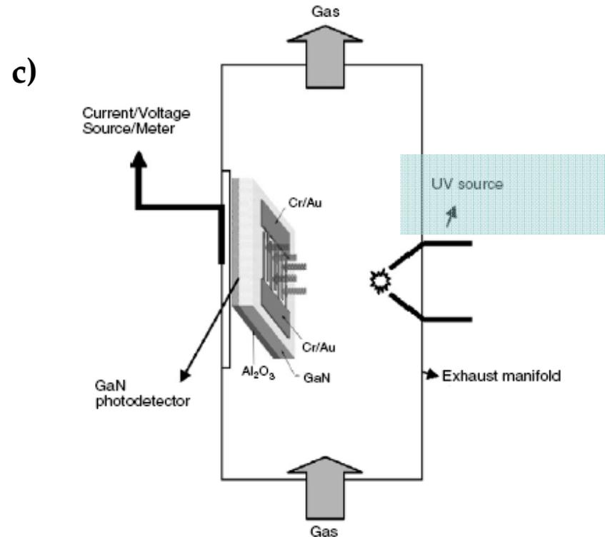
Schematic illustration of GaN based UV photodetector based gas sensor for auto-exhaust such as NO<sub>x</sub> and CO at temperature up to 550°C.
