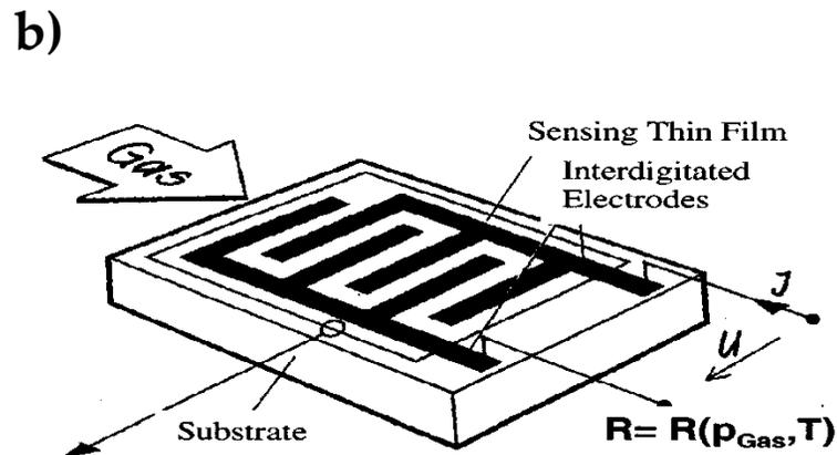
Typical structures of resistor-type gas sensors: a) tubular structure; b) interdigitative electrode (IDE) chip
