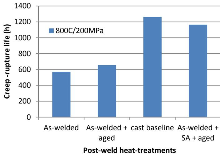
**Creep of cast HR 282 at 800C/200MPa**
