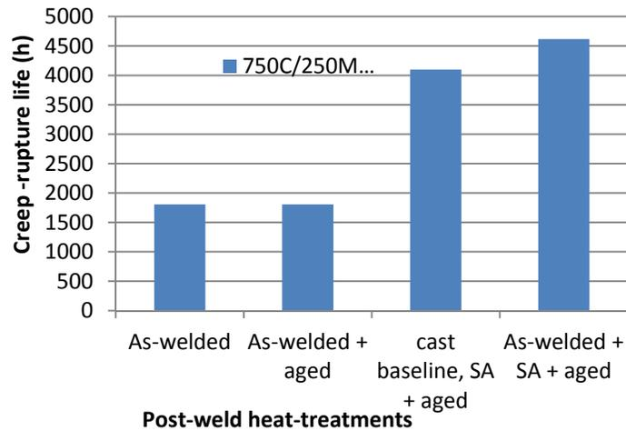
**Creep of cast HR 282 at 750C/250MPa**
