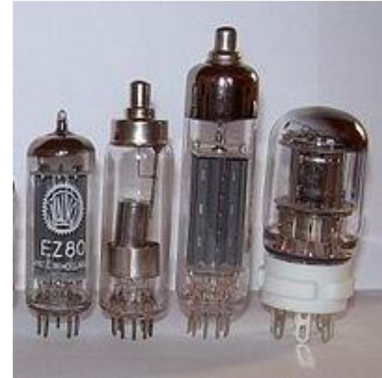
The 1946 [ENIAC](#) computer used 17,468 vacuum tubes and consumed 150 kW of power
