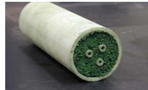
Thermocouple protection system for gasifiers (NETL website)
