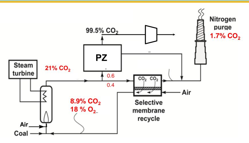
90% Capture Rate for the Entire System Absorption process removes 95% CO<sub>2</sub> from partial stream
