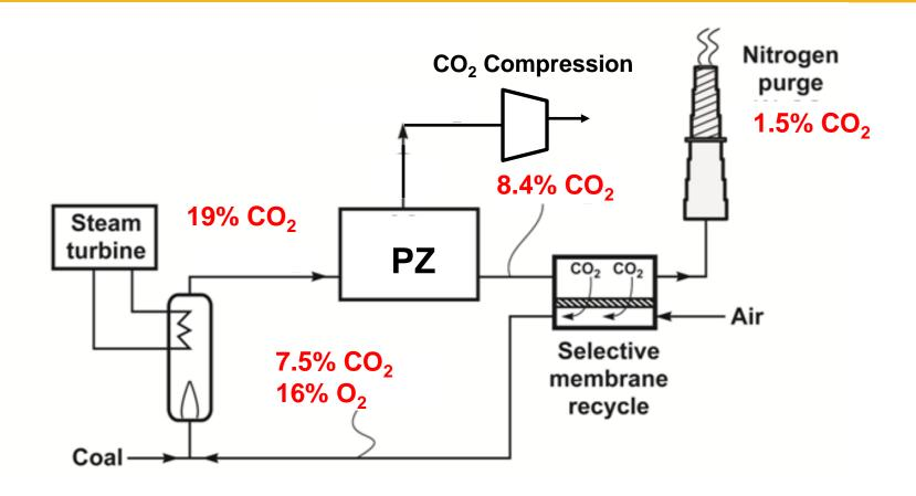
90% Capture Rate for the Entire System Absorption process removes 60% CO<sub>2</sub>.
