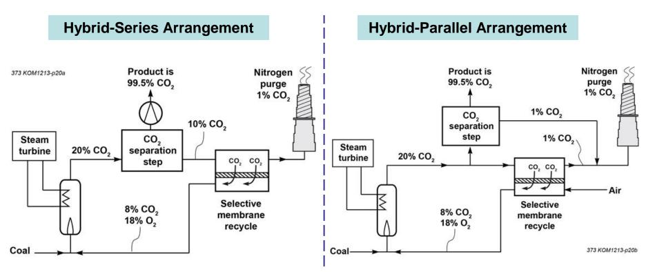
Depending on the arrangement, the selective recycle membrane can:
