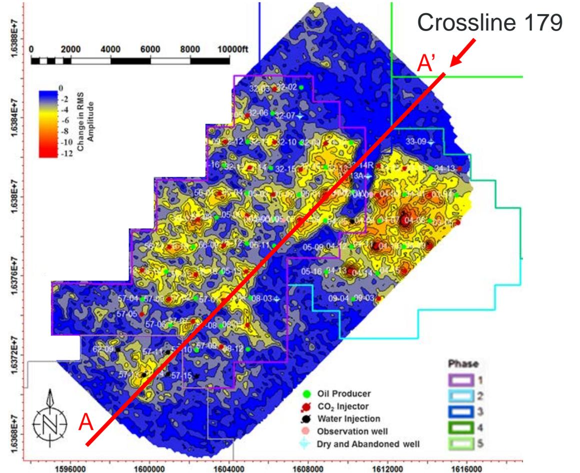
Time-lapse difference map of the reservoir displaying RMS amplitude changes.
