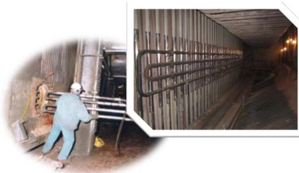
Fireside Corrosion (High-Sulfur Coal & In-Plant Testing)
