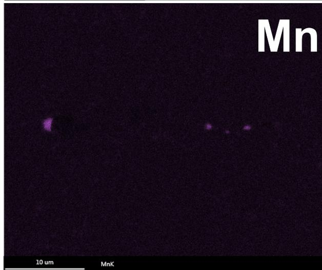
Just as in the simulated HAZ sample, damage is noted in the HAZ of cross-weld creep tests and associated with inclusions. There is a strong association of inclusions with Al and Ca; to a lesser degree with Mn. This is not surprising since this heat of Grade 92 has low sulfur (e.g. lower MnS can be expected)
