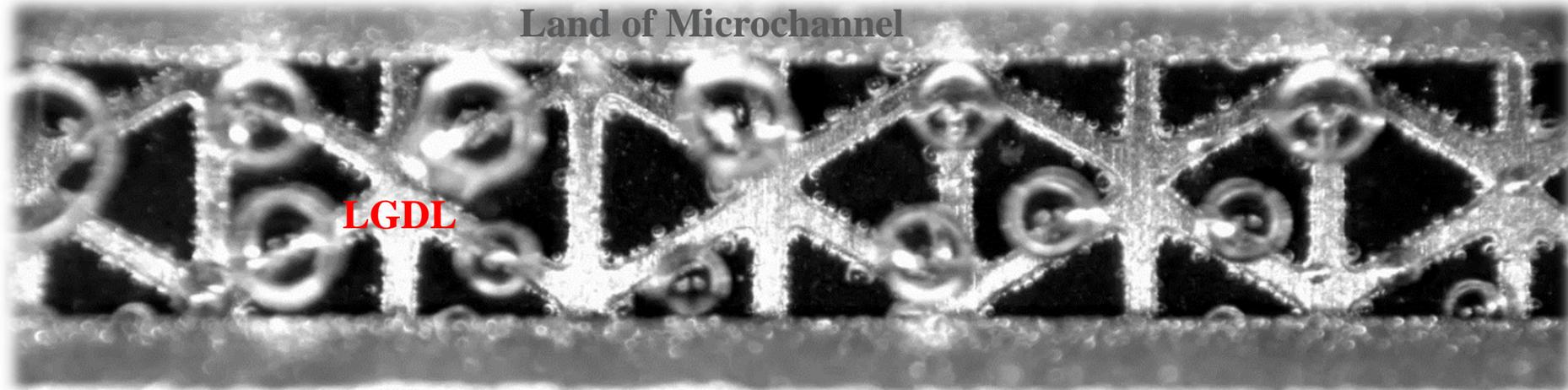
Deionized water full filled the microchannel and flow from right to left
